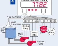
Relay #3 trips the High Level Alarm at 7500 gallons and resets at 6900 gallons.
