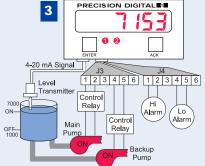
The backup pump is not able to keep up, so when the level reaches 7000 gallons, relay #1 transfers and starts the main pump.
